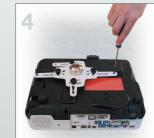
Fix the adjustable arm plate to the projector by positioning the plate's screws in correspondence to the designated holes on the bottom of the projector.
