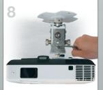
lock the 4 button screws ensuring that they are firmly fixed in order not to have any vibration or
